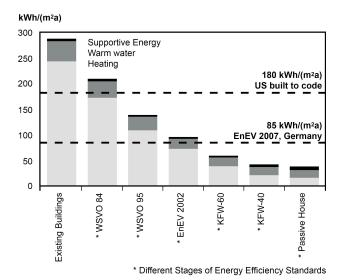
Figure 1: Energy-consumption of an average built-to-code building in the US and Germany
